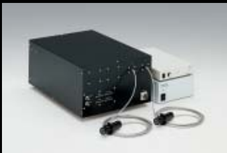
Dual Type The multi-combiner outputs laser light with two fibers. Light can be used both for observation and laser light stimulation.
