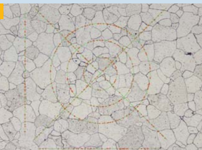
Horizontal, vertical, diagonal or circular measurement lines and combinations thereof are supported
