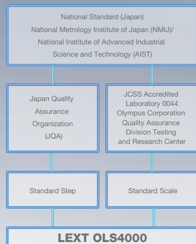
LEXT OLS4000 Traceability System Diagram
