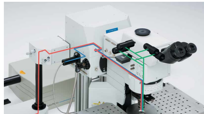
Red: IR pulsed laser, Blue: Visible light laser, Green: Fluorescent light
