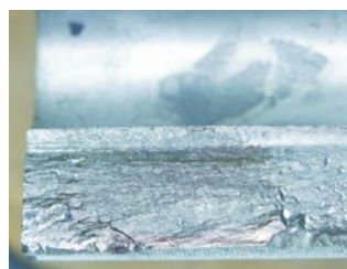
Four-part illumination of surface fracture (metal)
