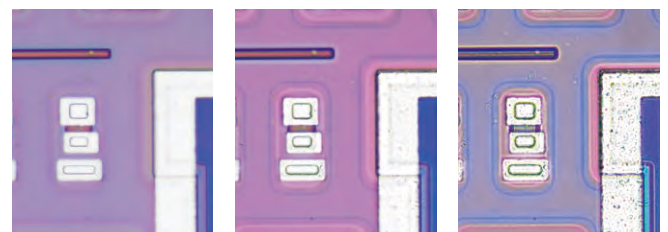
Minimum aperture: Higher contrast and larger depth of field
