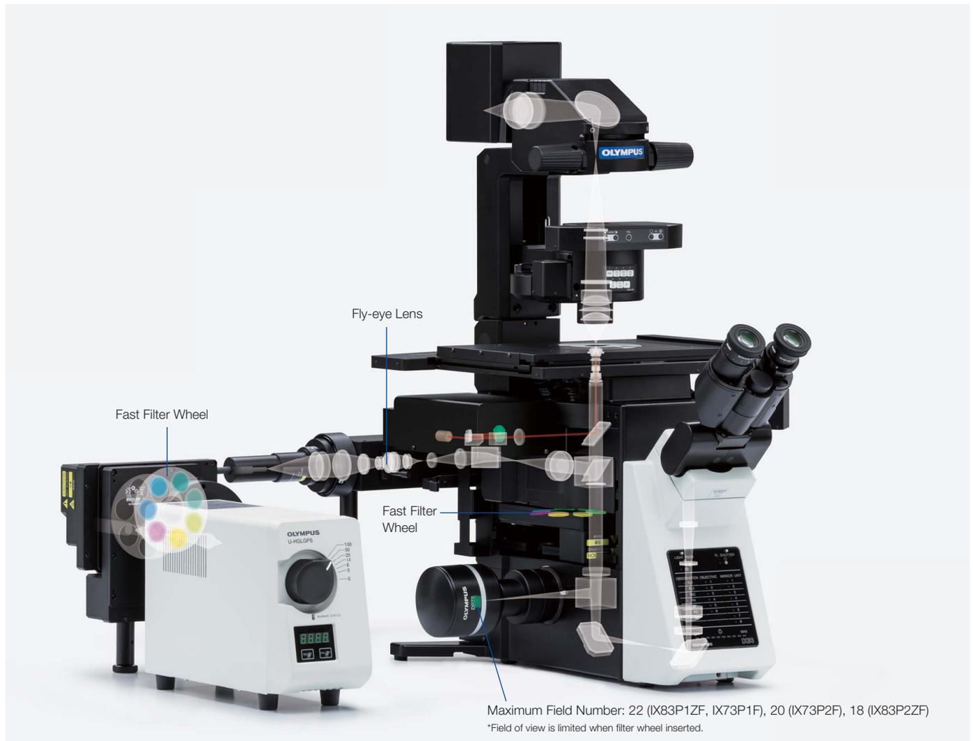
Olympus UIS2 infinity-corrected optics provide high optical transmittance with a broad range of objectives providing wide chromatic correction and high resolution, as well as high S/N primary images regardless of the observation method. The wide field of view and fly-eye lens system provide uniform fluorescence images and enable the use of sCMOS cameras with large sensors.
