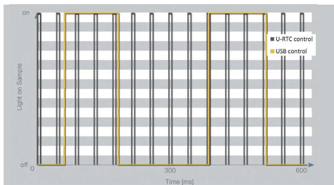
The precision and speed (i.e. images taken per time) of experiment set-ups is more accurate and faster when the experiment is controlled via the RTC (blue) compared to PC control only (orange). Measurements were performed by using Lumen Dynamics XLED1 light source, Andor iXON 897 EMCCD camera, and a light meter at the objective lens. Data were acquired with 5 ms exposure running the camera as fast as possible.
