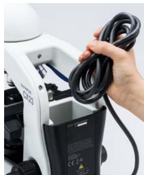
Cable storage compartment
